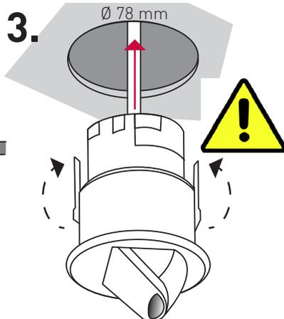
Insert the detector into the cutout. Take special care when bending the springs back
