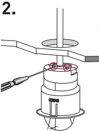
Attach the cable clamp.
