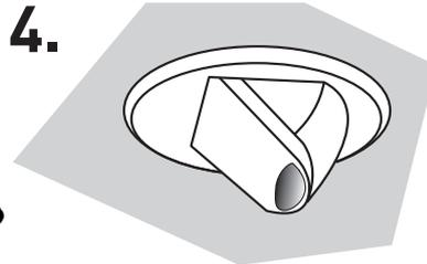
Ensure the fitted unit sits flush to the ceiling.
