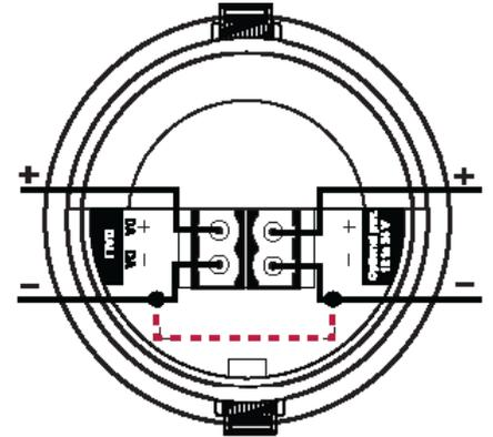
link between the DALI negative terminal and the negative terminal of the external power supply, as shown in the figure.
