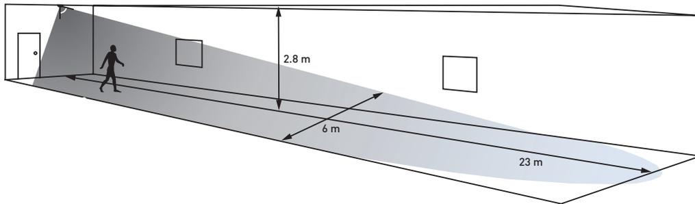
Detector head position at 80° to the vertical for large offices or classrooms, and for corridor and aisles. Sensitivity set to maximum.
