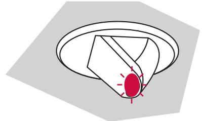
With the circuit switched on the LED in the sensor will flash red for 30 seconds.
