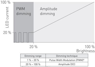
\* PWM dimming frequency 800 Hz
