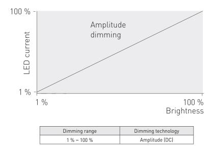
LC27MINI-FD-150-700 LED driver implements amplitude dimming technology across whole dimming range. Amplitude dimming offers the best available technology for dimming the light output in an accurate and flicker-free way to ensure high quality lighting in even the most demanding situations such as camera recording applications. Amplitude dimming technology complies with IEEE 1789-2015 recommendations of current modulation to mitigate health risks to viewers.
