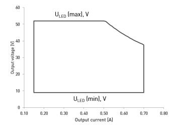
Note: 1) Dimming between 1 % - 100 % possible across the operating window, restricted by the absolute minimum dimming current of 5 mA.
