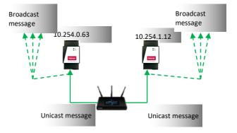
Tip!IP Routers do NOT permit broadcast messages. A BBMD (BACnet Broadcast Message Device)<br/>sends a unicast message to the specified BBMD device on the other subnet range.
