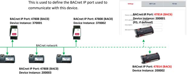
Caution Ensure a unique 'Network number' is configured for each 436 Interface/Report on the BACnet IP network and all devices that need to communicate with each other are using the same 'BACnet IP Port'.
