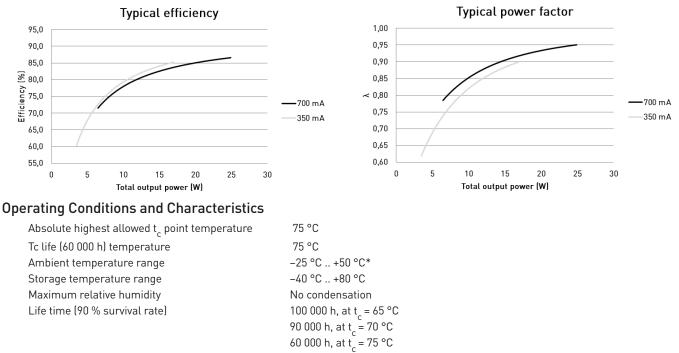
\*) For other than independent use, higher t<sub>a</sub> of the controlgear possible as long as highest allowed t<sub>a</sub> point temperature is not exceeded
