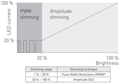
\* PWM dimming frequency 800 Hz
