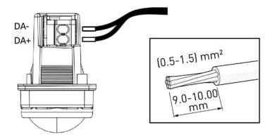
Note: To remove DALI wiring, press down the release buttons.
