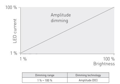
LC44MINI-DA-700-1050 LED driver implements amplitude dimming technology across whole dimming range. Amplitude dimming offers the best available technology for dimming the light output in an accurate and flicker-free way to ensure high quality lighting in even the most demanding situations such as camera recording applications. Amplitude dimming technology complies with IEEE 1789-2015 recommendations of current modulation to mitigate health risks to viewers.
