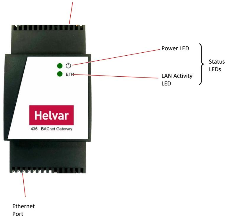
**Note:** Typically, individual systems (energy control, lighting, boiler and air-conditioning systems, etc.) are measured separately for CO<sub>2</sub> accountability. Therefore, installing the BACnet Gateway and combining the various systems can help an effective BeMS be more energy efficient and comply with national building regulations.
