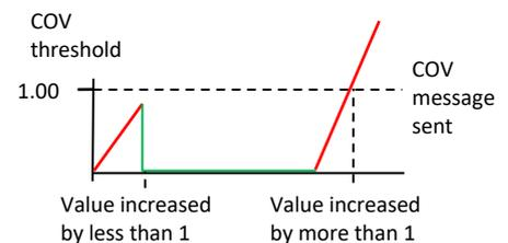
**Note:** Typically, BACnet servers wait for a BACnet client to request data before responding, but this optional BACnet property sends a COV message when the COV threshold is exceeded.
