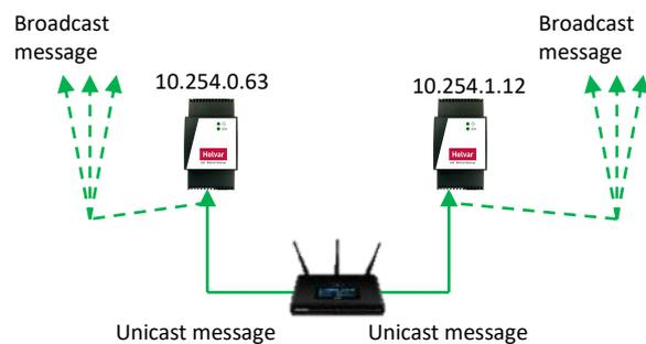
**Tip!** IP routers do NOT permit broadcast messages. A BBMD (BACnet Broadcast Message Device) sends a unicast message to the specified BBMD device on the other subnet range.
