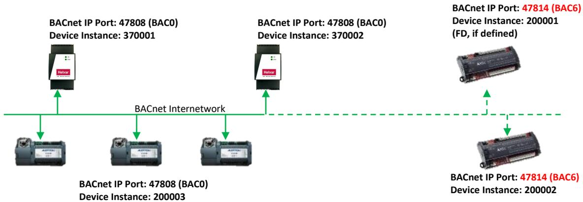
**Caution** Ensure a unique 'Network number' is configured for each 436 Interface/Report on the BACnetIP network and all devices that need to communicate with each other are using the same 'BACnetIP Port'.
