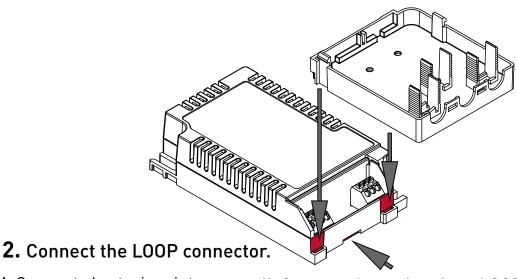
I. Connect short wires into LOOP connector (depending on the amount of input terminals in LED driver)
