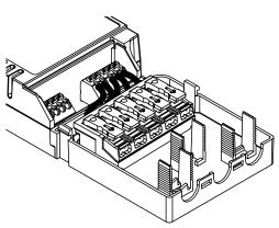
3. Connect wires into correct terminals according to driver datasheet instructions, both into LOOP connector and into LED load connector.
