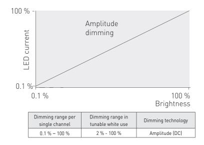
LC45iC-DA-100-900 LED driver implements amplitude dimming technology across whole dimming range. Amplitude dimming offers the best available technology for dimming the light output in an accurate and flicker-free way to ensure high quality lighting in even the most demanding situations such as camera recording applications. Amplitude dimming technology complies with IEEE 1789-2015 recommendations of current modulation to mitigate health risks to viewers.
