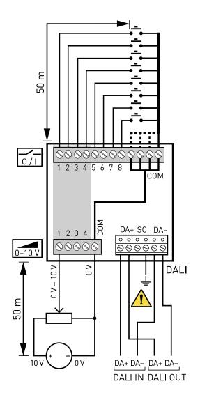
**Note:** To avoid interference, do not install close to high current switching devices. Keep the input wiring as short as possible. Use shielded cable, if necessary.
