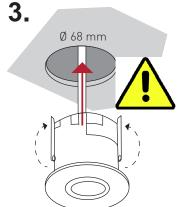
Insert the detector into the cutout.Take special care when bending the springs back
