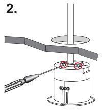
Attach the cable clamp.
