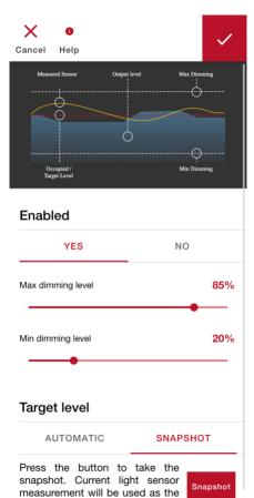
Purpose of the daylight harvesting (DLH) is to reduce the usage of artificial light when natural light is available. Light sensor measures the amount of light reflecting from the surface right below the sensor, so the luminaire can respond to the amount of natural light in the space by dimming the light, which helps to save energy and at the same time maintain the lighting level optimal for the user.
