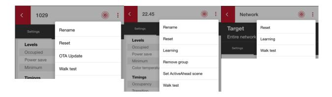
You can find walk test under node, group and network pages' three dots menu. Walk test will force the targeted nodes to go to unoccupied state using the configured fade down time. In case movement is detected, the nodes will immediately react to it and fade up to occupied light level. Consequently, walk test requires the space to be empty. No one else should move there and disturb your test process.
