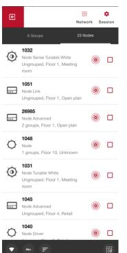
"Main screen" is the central view to navigate through the nearby nodes and groups in the connected network. Here you can find a tab with a list of the discovered nodes and another tab with a list of discovered groups. Filtering options are located at the bottom of the view.
