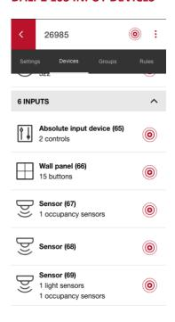
DALI-2 103 input devices will show up in the input device list, where they can be identified.
