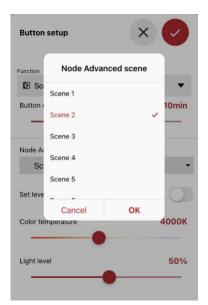
**Note:** Node Advanced requires selecting a DALI scene to be used with the Scene button. **DALI scenes are device specific, not button specific,** which means that light level and colour temperature modifications apply also to other buttons which have the same DALI scene configured.
