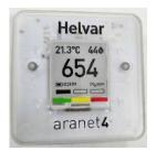
Currently only one type of extension sensor is supported – Aranet4. To link it to Environmental sensor, open the Environmental sensor page in Mobile App.
