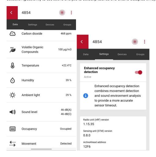
Environmental sensor can be added to a group of ActiveAhead nodes and notify the group about movement when it is detected, so the group lights can react. This is only ActiveAhead grouping, not related to Imagine system. Environmental sensor cannot be used for Daylight Harvesting yet.
