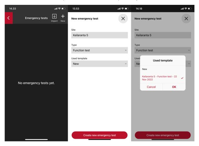
Select "New." if you want to create a new test. Write the site name and select the test type (function or duration). Next, choose a template if you have previously completed tests from the same site. This is how all emergency devices, which were found during the previous test, are transferred from the template to the new test. We recommended to use the most recent completed test as the template to ensure that every device in the site gets tested. Finally, press "Start a new emergency test".
