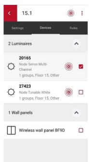
Daylight harvesting function is enabled by default on individual luminaires. To achieve an evenly dimmed ceiling, a group daylight harvesting master can be selected.
