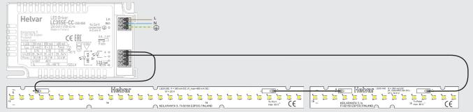
1x LS-562-3100lm + 1 x LS20-142-800lm modules connected with Helvar LL35HE-CC-120-450 LED driver at 350 mA driving current
