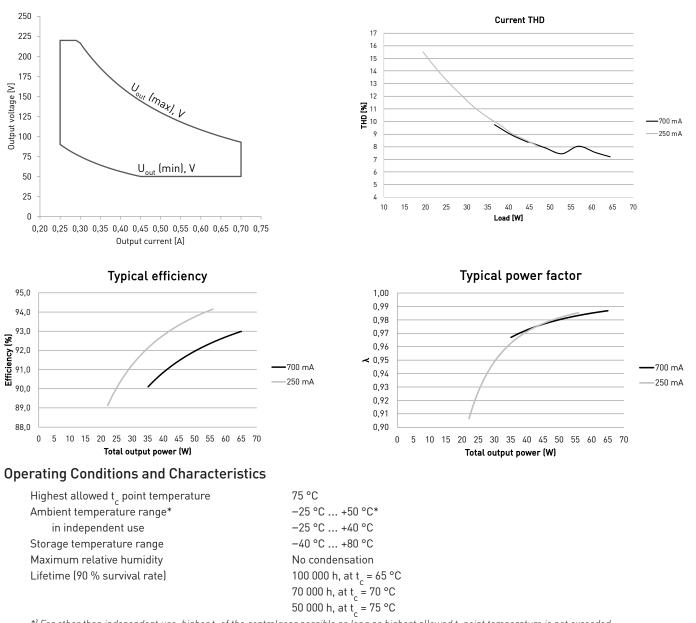
\*) For other than independent use, higher t<sub>a</sub> of the controlgear possible as long as highest allowed t<sub>c</sub> point temperature is not exceeded
