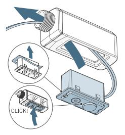
3. Feed the cable through the hole in the luminaire. Connect the cable to the Node. Fasten the holder to the luminaire using the O-ring and a M20 nut.
