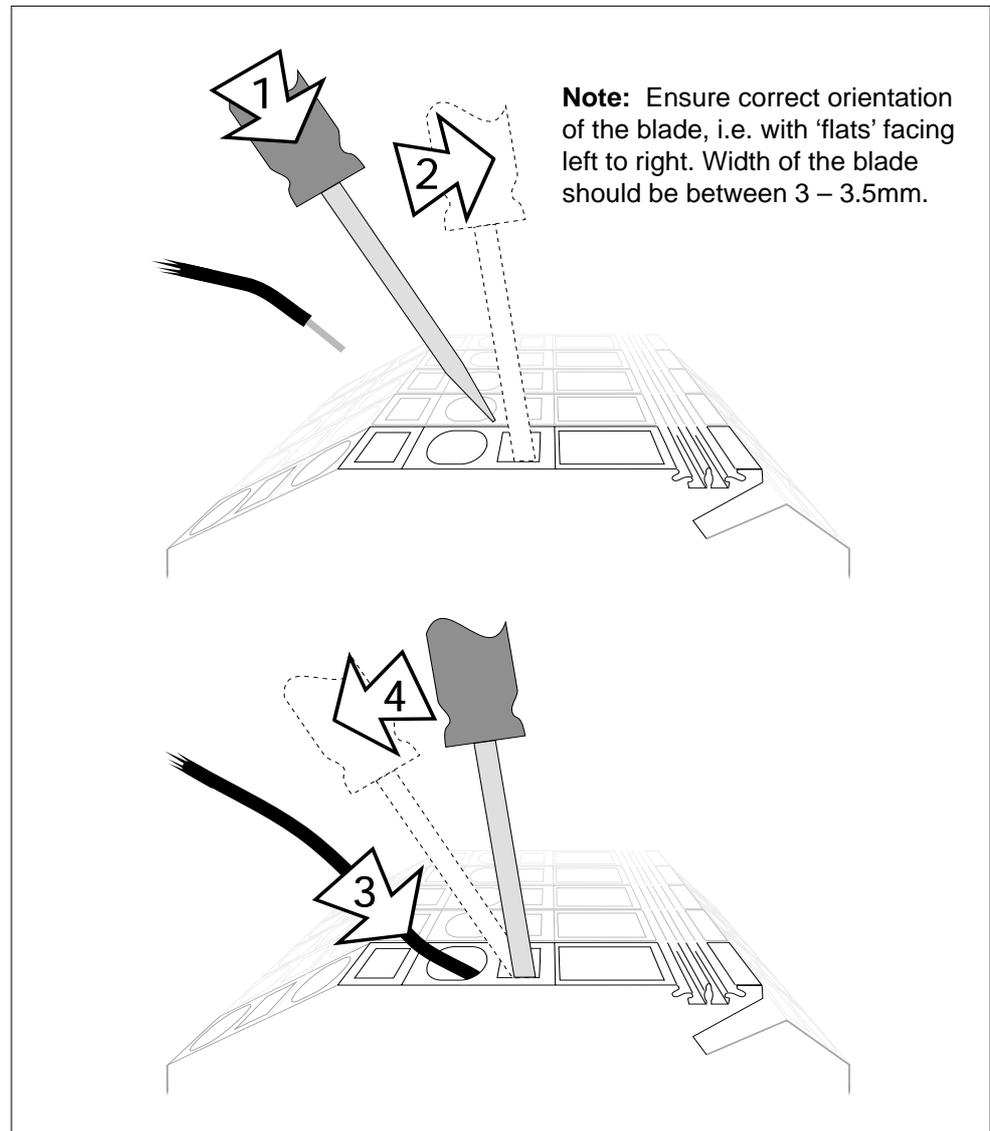
Fig.4-2: Connecting to 'cage-clamp' output terminals.
