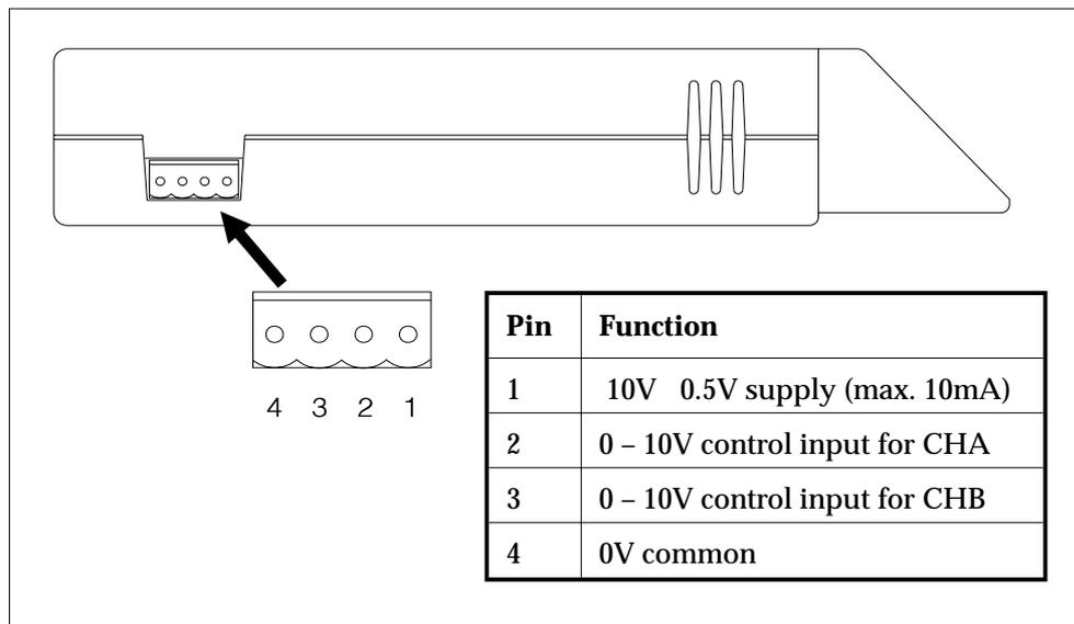
Fig.6-1: Analogue input connector.
