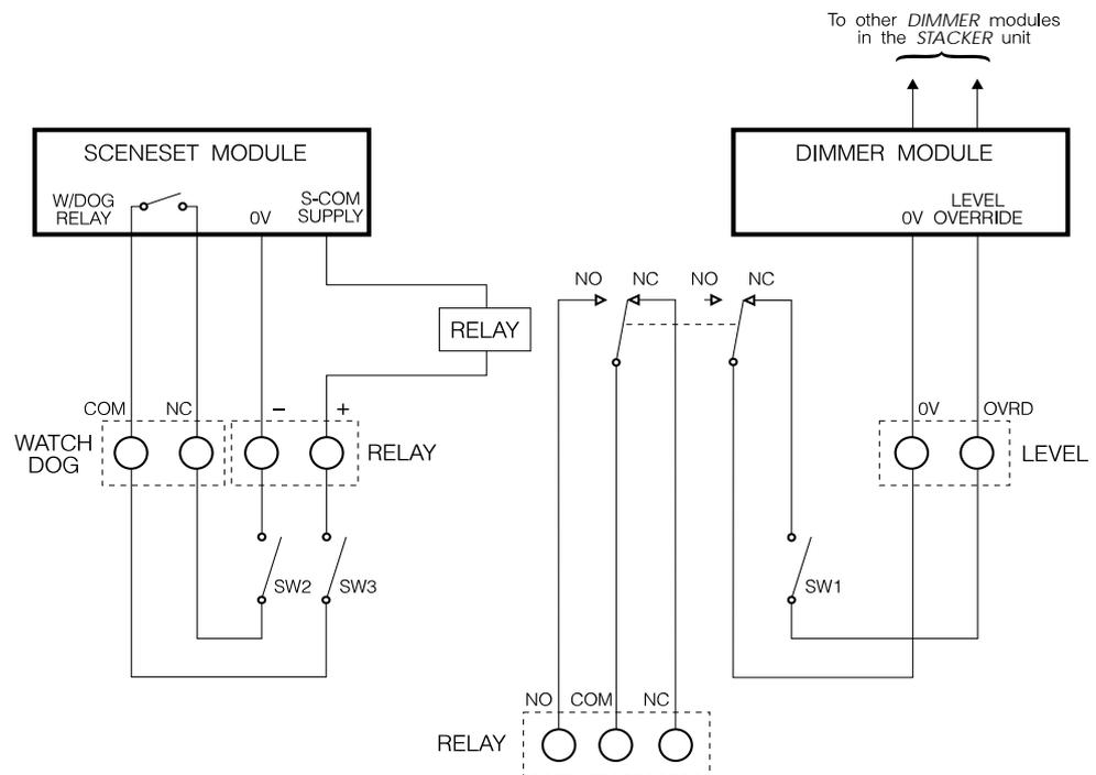
Fig.5-8: Watchdog and level override circuit details.
