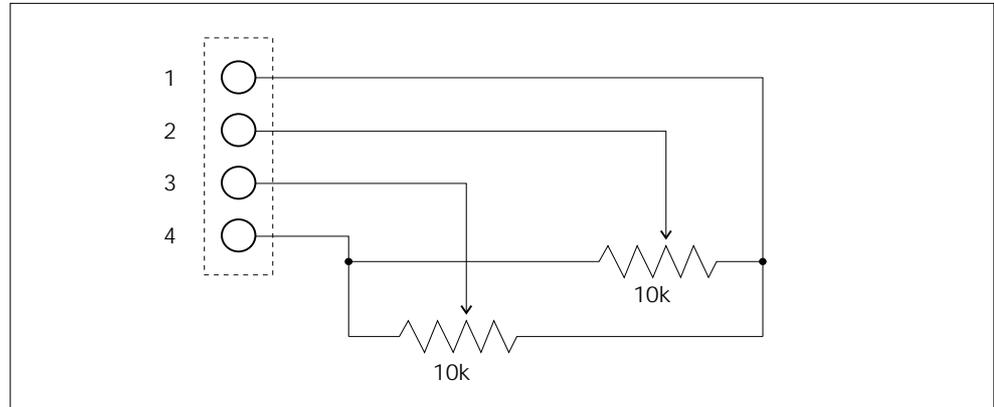
*Fig.6-2: Basic analogue control circuit.*
