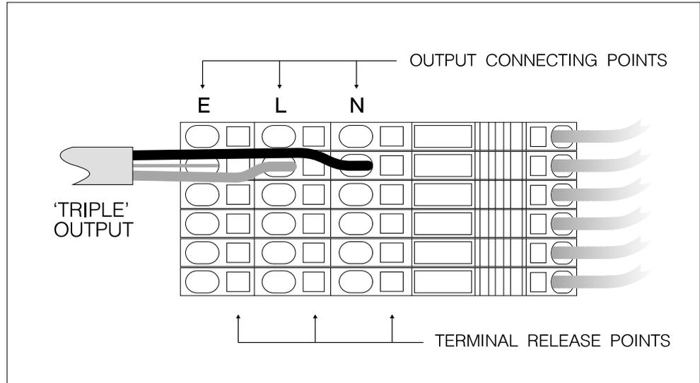
Fig.4-1: Power output connections.
