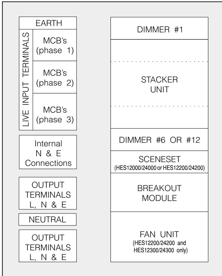
Fig.1-1: Internal layout of Pre-wired Cabinets.
