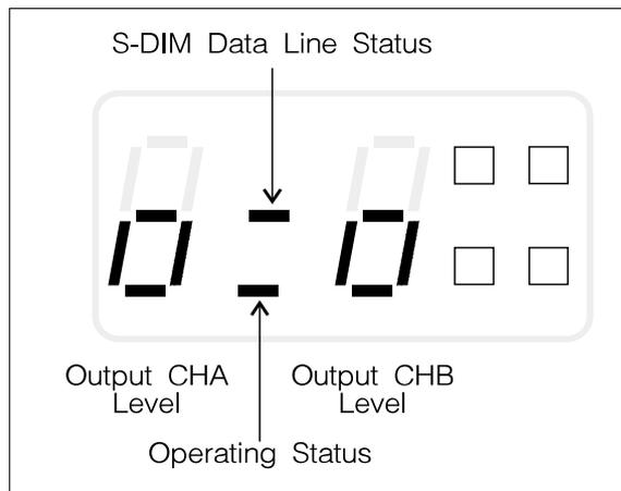
Fig.8-2: Channel level mode display.
