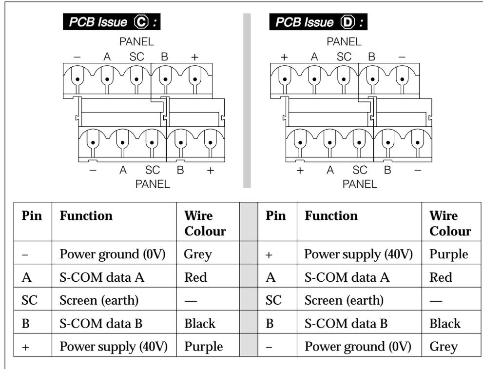
Fig.5-3: Connection details for S-COM (external).
