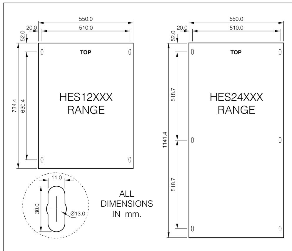
Fig.2-2: Dimensions of cabinet rear fixing holes.
