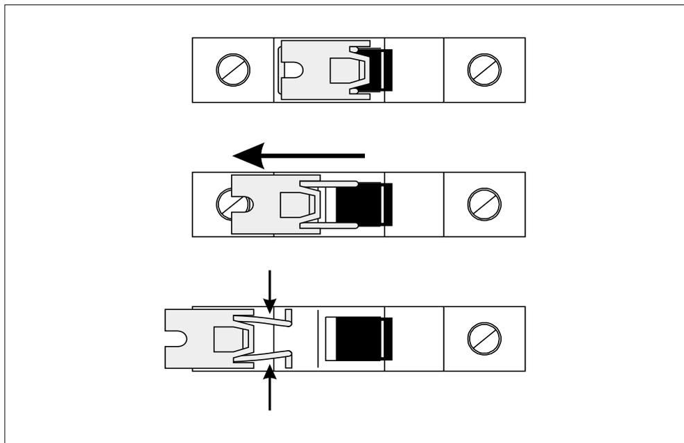
Fig.3-5: Removing the MCB anti-tamper clip.
