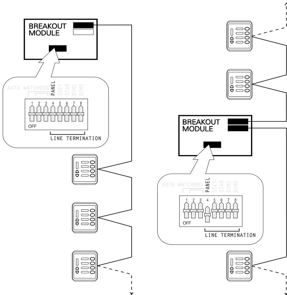
Fig.5-4: S-COM termination on BREAKOUT Module.
