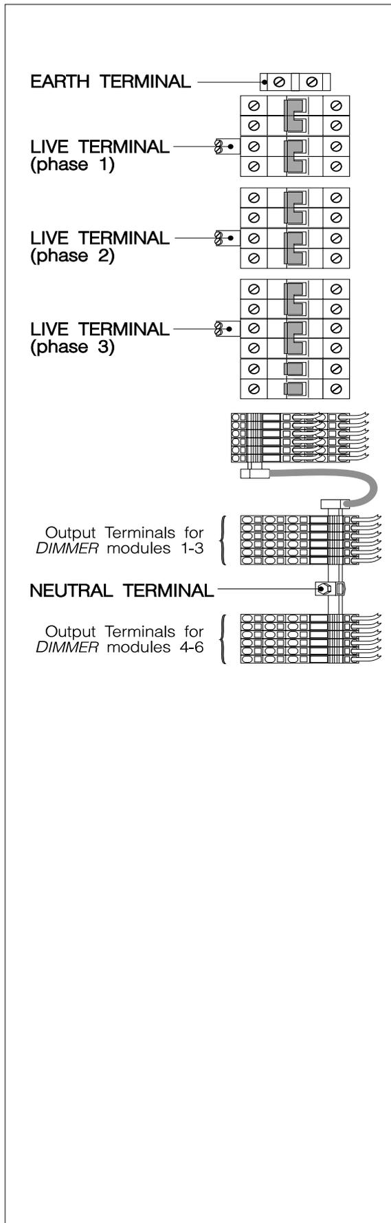
Fig.3-1: Main input terminals for HES12xxx range.
