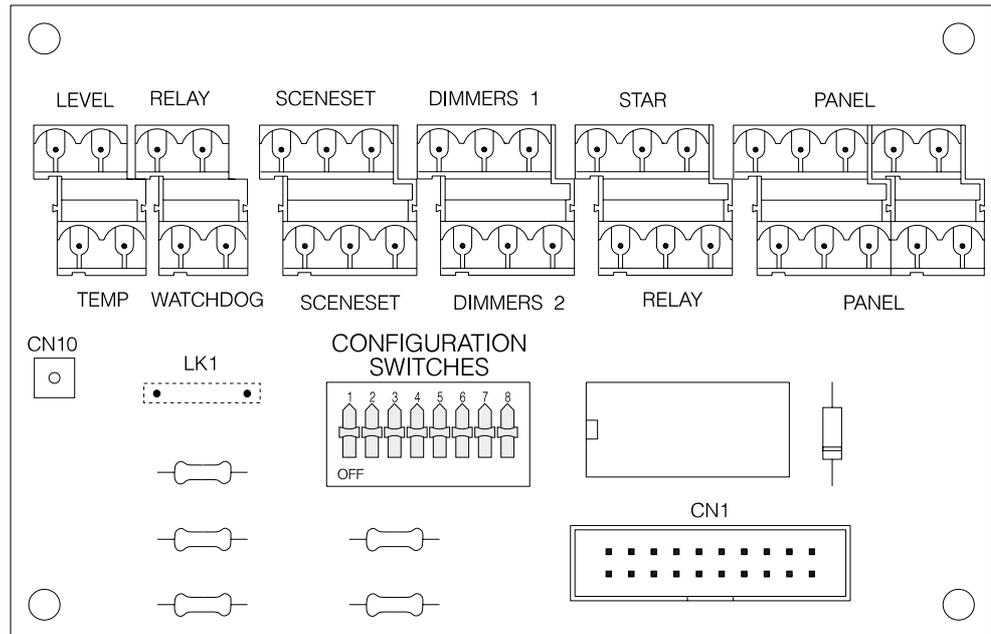
Fig.5-1: Layout of BREAKOUT module.
