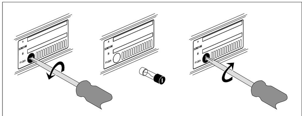
*Fig.11-2: Removing the S-COM supply fuse.*
