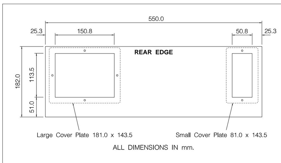
Fig.2-6: Cable entry cut-out and plate dimensions.
