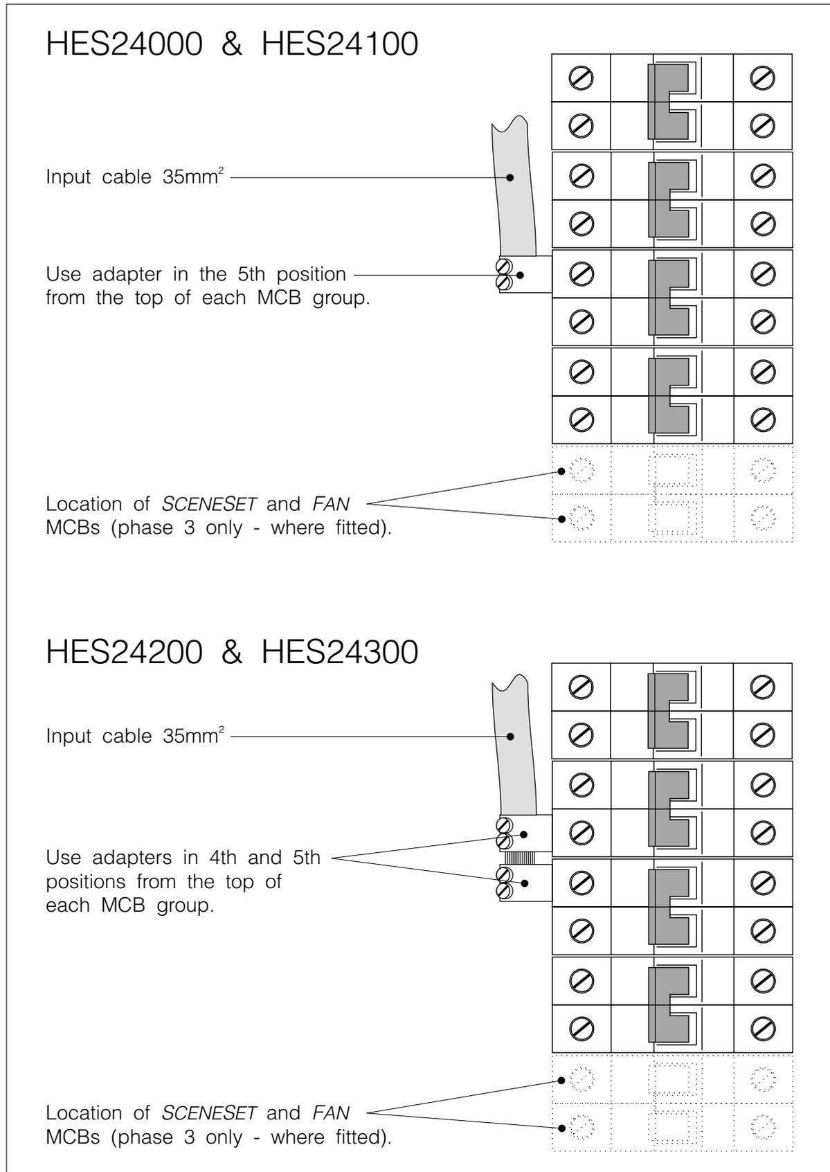
*Fig.3-4: HES24xxx range - live input connections.*
