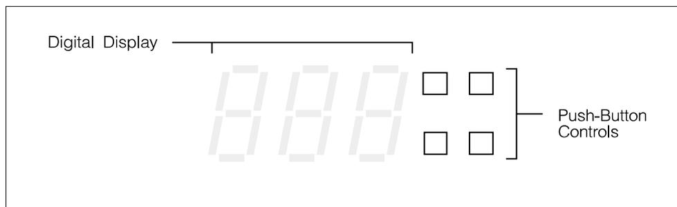
Fig.8-1: *DIMMER* control panel.
