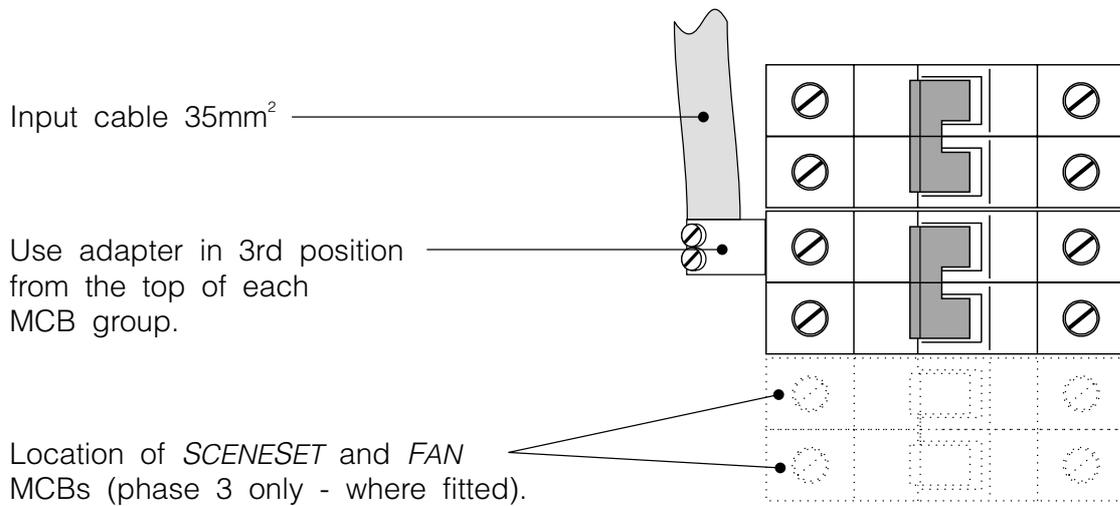
Fig.3-3: HES12xxx range - live input connections.
