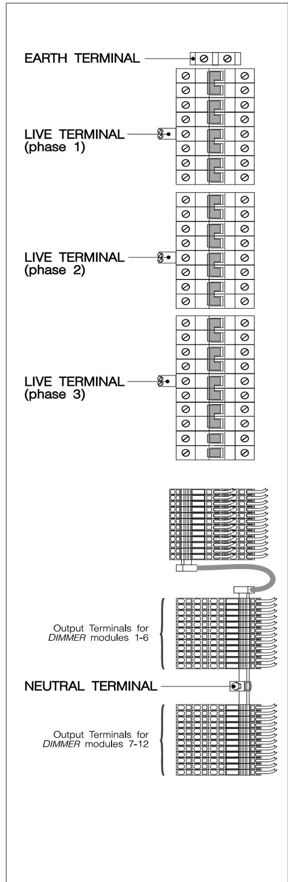
Fig.3-2: Main input terminals for HES24xxx range.
