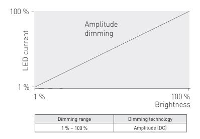
LL35SE-DA-250-850 LED driver implements amplitude dimming technology across whole dimming range. Amplitude dimming offers the best available technology for dimming the light output in an accurate and flicker-free way to ensure high quality lighting in even the most demanding situations such as camera recording applications. Amplitude dimming technology complies with IEEE 1789-2015 recommendations of current modulation to mitigate health risks to viewers.
