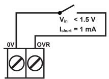
To provide output level override functionality, wire a switch between the '0 V' and '0VR' terminals.
