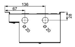
Knockouts: base (for power and output cables)
