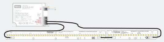
1 x LX-562A + 1 x LX-142A modules connected with Helvar LL1x10-42-CC-350-700 LED driver at 450 mA driving current
