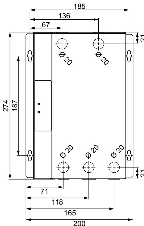
Knockouts: base (for power and output cables)
