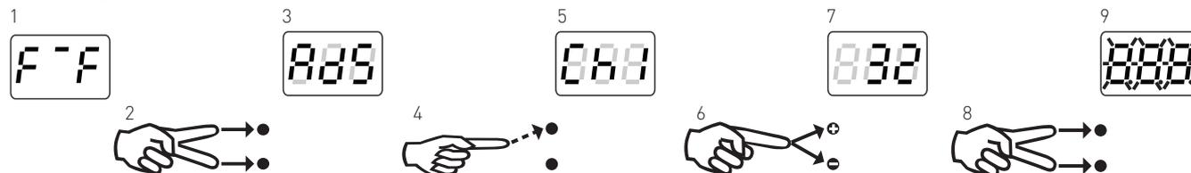
With the status display (1) showing, press and hold both buttons (2) to step through the menu. When the display shows AdS (3), press the top button once (4) to display Chl. When Chl is shown (5), press and hold one of the buttons (6) until the required address value is shown (7: this example is 32). Press both buttons (8) to store the setting. The display flashes 888 when the value is stored (9).
