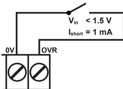
To provide output level override functionality, wire a switch between the '0 V' and 'OVR' terminals. Switch closure sets the light output of the dimmer channel to the override level.
