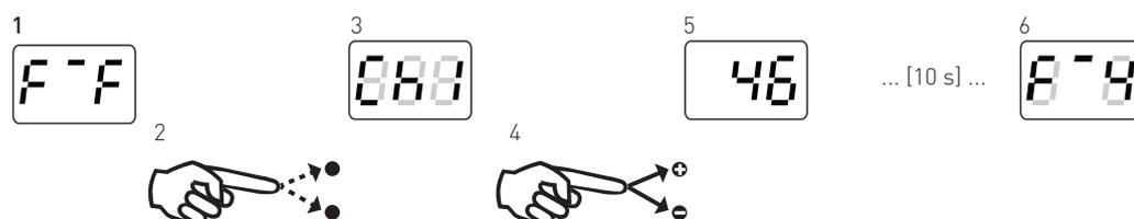
With the status display (1) showing, press either button once (2) to display REL or Chl (3). Press and hold the top or bottom button (4) to adjust the level. When the required level is reached (5: this example shows 46 %), release the button.
