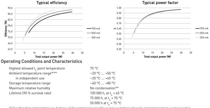
\*) For other than independent use, higher t<sub>a</sub> of the control gear possible as long as highest allowed t<sub>a</sub> point temperature is not exceeded \*\*) Coated version: partially allowed condensation,  $T_a = -40.. +50 \ ^\circ C$
