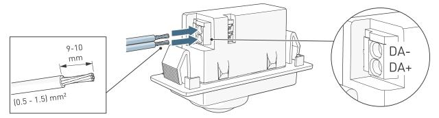
Note: To remove DALI wiring, push down the release buttons.
