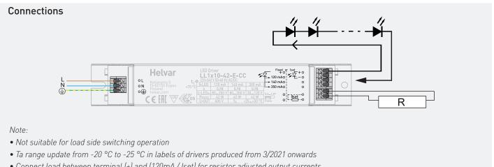
• Connect load between terminal (+) and (120mA / Iset) for resistor adjusted output currents.
