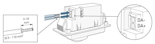
Note: To remove DALI wiring, press down the release buttons.
