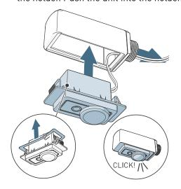
3. Feed the cable through the hole in the luminaire. Connect the cable to the Node. Fasten the holder to the luminaire using the 0-ring and a M20 nut.
