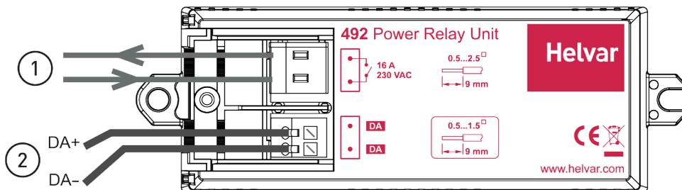
1. Load (relay) wiring
