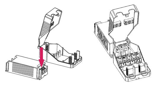
2. Connect L/N cables in on /off & Freedom models and L/N/DA1/DA2 cables in DALI models to the 5-place connector. Ensure that the cables are firmly and securely mounted into the connector!
