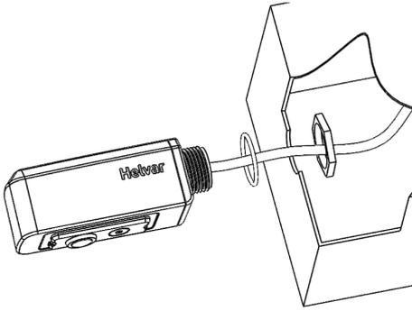
d) Feed the cable through the hole in the luminaire, connect the cable to the LED driver and fasten the holder to the luminaire using the O-ring and a M20 nut.
