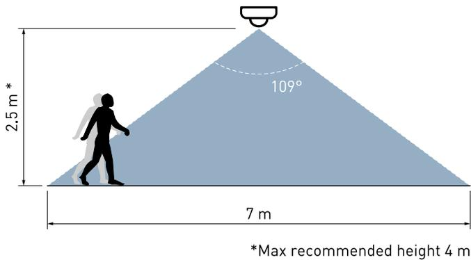
Detection pattern at floor level for 2.5 m mounting height
