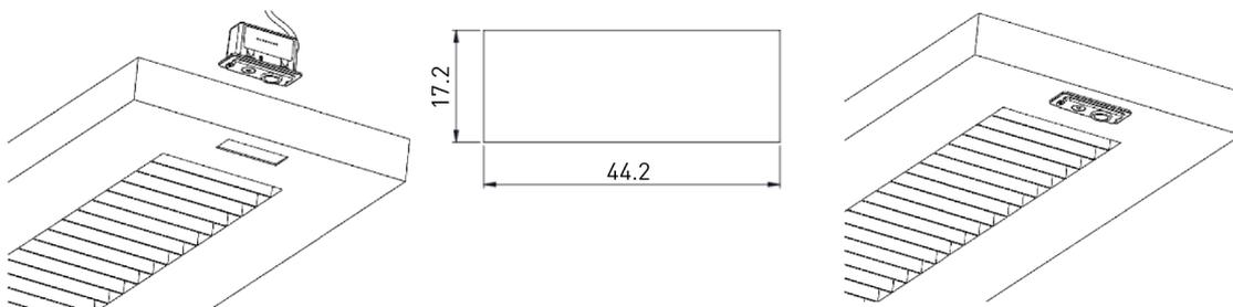
Ensure the face of the unit sits level with the luminaire casing and secure the unit in place.
