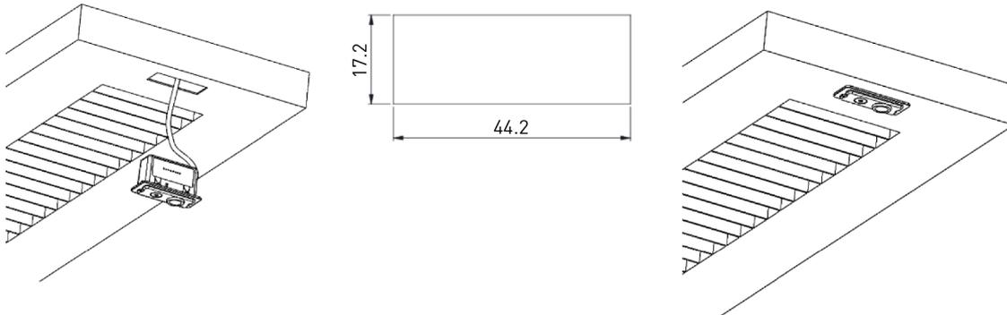
Carefully push the unit into the cutout until it 'clicks' into place and sits flush with the luminaire casing. Supported luminaire frame thickness in the range  $0.4 \leq d \leq 1.5$  mm.
