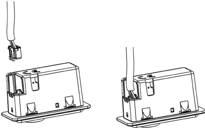
5635 Multisense has a connector for the Freedom connecting cable.
