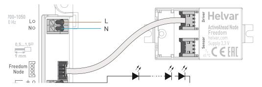
Note: Ensure connectors securely 'click' into place when plugged in correctly.
