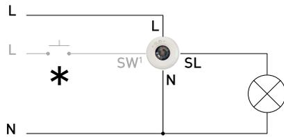
\*: Mains-rated retractable wall switch ~230 VAC
