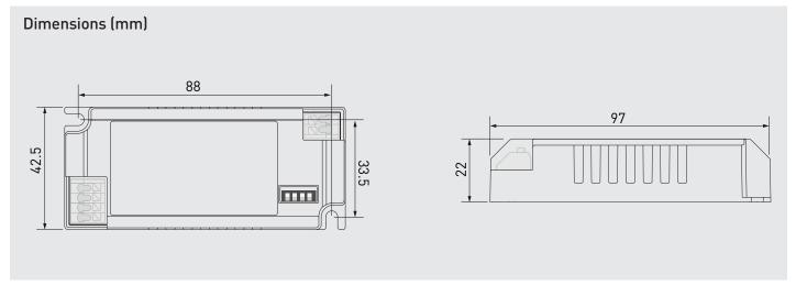
In LC26MINI-DA-250-700, the current can be set with dip-switches. With each combination of switch setup, a different output current value can be set. The maximum value can be reached with all switches set to "1" (pushed downwars, away from the connectors, see connections picture above) and minimum with all switches set to "0" (pushed upwards, towards the connectors). The output current values according to the dip-switch settings are presented below.
