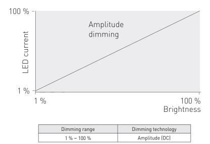
LC26MINI-DA-250-700 LED driver implements amplitude dimming technology across whole dimming range. Amplitude dimming offers the best available technology for dimming the light output in an accurate and flicker-free way to ensure high quality lighting in even the most demanding situations such as camera recording applications. Amplitude dimming technology complies with IEEE 1789-2015 recommendations of current modulation to mitigate health risks to viewers.
