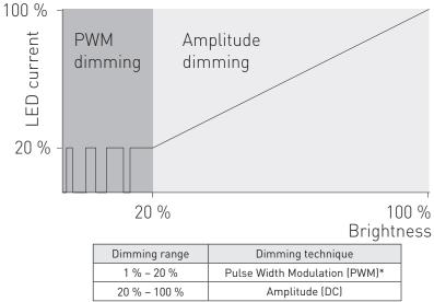
PWM dimming frequency 1 kHz
