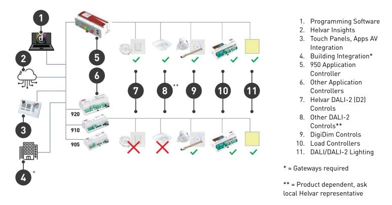
Compatibility: DALI and DALI-2 Lighting (Control Gear), DigiDim Controls, NOT DALI-2 (D2) controls (Control Devices)
