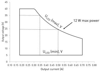
Note: Dimming between 1 % - 100 % possible across the operating window, restricted by the absolute minimum dimming current of 3 mA.
