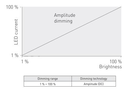
LC12TINY-DA-180-700 LED driver implements amplitude dimming technology across whole dimming range. Amplitude dimming offers the best available technology for dimming the light output in an accurate and flicker-free way to ensure high quality lighting in even the most demanding situations such as camera recording applications. Amplitude dimming technology complies with IEEE 1789-2015 recommendations of current modulation to mitigate health risks to viewers.
