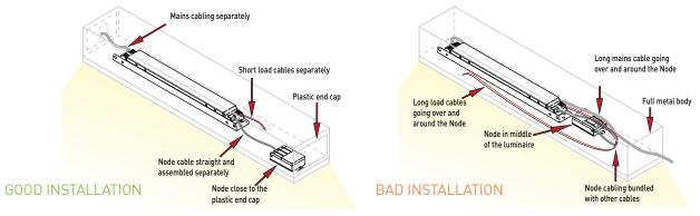
When the Freedom Node is installed inside luminaire with the driver, the following things needs to be taken in consideration regarding the communication:
