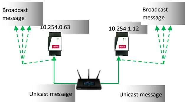
**Tip!** IP Routers do NOT permit broadcast messages. A BBMD (BACnet Broadcast Message Device) sends a unicast message to the specified BBMD device on the other subnet range.
