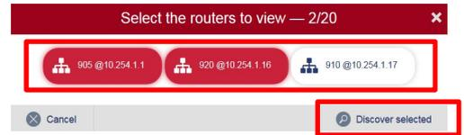
6. Press **Discover selected** to detect all Router and the devices connected to the available Router subnets. This will display the network tree associated with the selected workgroup.
