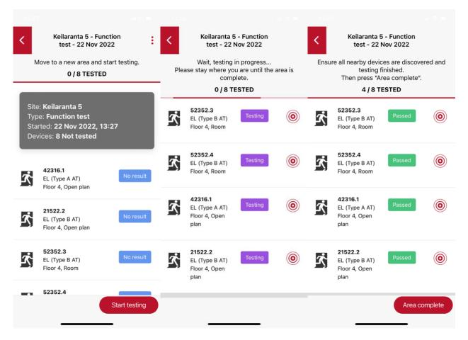
**Note:** Always keep the application at foreground during testing. Avoid moving since it may break the connection to the proxy node.
