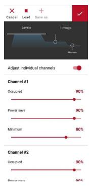
Luminaires built with the Helvar Freedom Dual Channel LED drivers can be used in two channel mode. In the most common use case, one channel is for the indirect light i.e "uplight" and the other for the direct light i.e "downlight".
