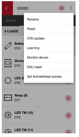
DALI reset can be started with the AAG2 App to force Node Advanced to clear its memory, re-address and re-initialize DALI devices and DIGIDIM sensors attached to its DALI bus. This can be done through the three dots in the top-right corner of the node details screen, by selecting "DALI reset" in the menu.
