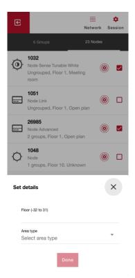
It is possible to set floor and area type for multiple nodes at once. You can do this by first selecting the nodes,
