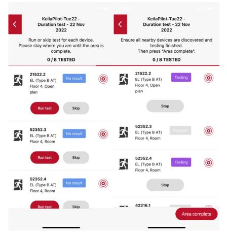
When the tests have completed, you need to collect the results. To do that, use the same locations where you have started the tests if possible. Select the ongoing test from the "*Emergency tests list*" and press "Continue." The app will automatically fetch the results for the nearby devices which have finished the test, but again you need to take care of starting the test for devices which were previously skipped.
