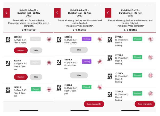
After the tests have run for the remaining devices, you will need to return to the site one final time to gather the results. At this point, all devices should be now tested.
