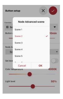
**Note:** Node Advanced requires selecting a DALI scene to be used with the Scene button. **DALI scenes are device specific, not button specific,** which means that light level and colour temperature modifications apply also to other buttons which have the same DALI scene configured.
